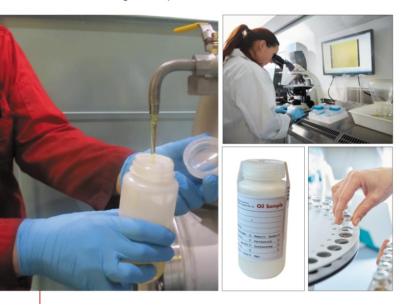
Oil Monitoring and Inspection Program (OMP) includes: Oil sampling – Oil analysis – Filter condition – Annual Inspection – Pre-Docking Inspection
